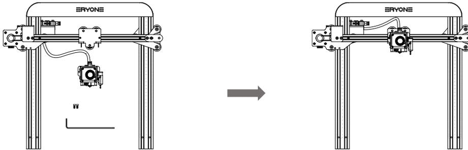
**3. Assemble the Gantry Frame:** Prepare the gantry frame parts, base, M5X35 round head hexagon socket screw x 4, M5 hex key allen wrench.
