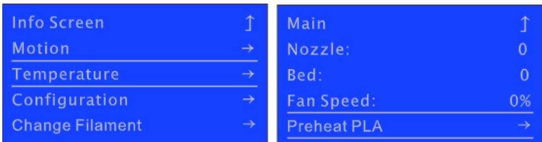
Choose “Motion” → “Disable Stepper”. After unlocking the motor, we move it to the center of the X axis.
