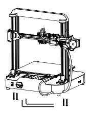
Insert the lead screw and tighten the screw
