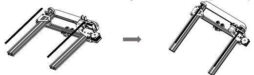
**2. Assemble the Extruder:** After assembling the gantry frame parts, take out your M3X6 screws, use the hex key allen wrench to fix the extruder.
